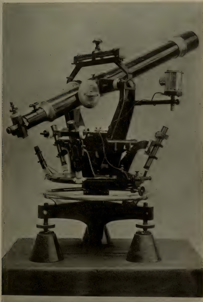
FIG. 27. Twelve-inch Theodolite. (Coast and Geodetic Survey.)
